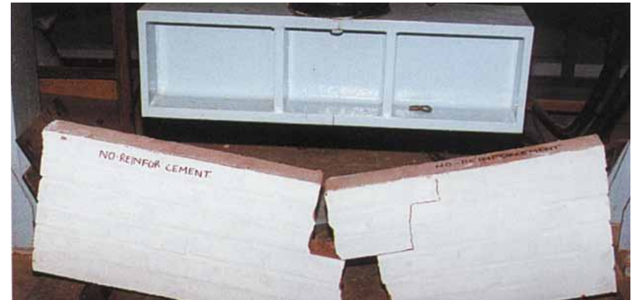
Destruction testing of un-reinforced wall
